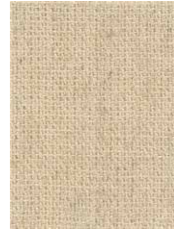
No. 7, 9 経糸, 緯糸: バナナ50%×綿50% 混紡糸 warp, weft: 50/50 banana/cotton blended yarn
