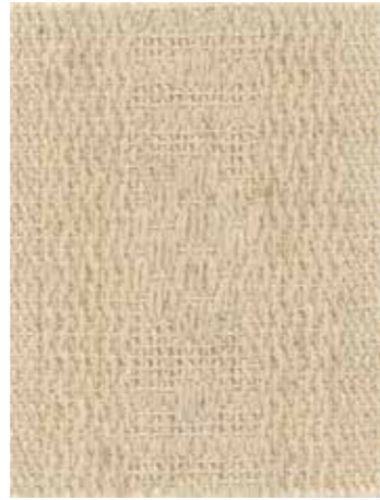
No. 1 経糸, 緯糸: バナナ50%×綿50% 混紡糸 warp, weft: 50/50 banana/cotton blended yarn
