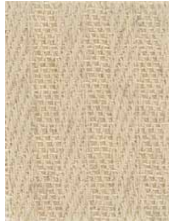
No. 3, 4 経糸, 緯糸: バナナ50%×綿50% 混紡糸 warp, weft: 50/50 banana/cotton blended yarn
