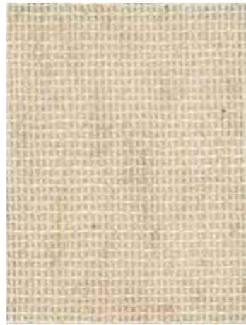
No. 5 経糸: バナナ50%×綿50% 混紡糸 緯糸: バナナ50%×絹50% 混紡糸 warp: 50/50 banana/cotton blended yarn weft: 50/50 banana/silk blended yarn
