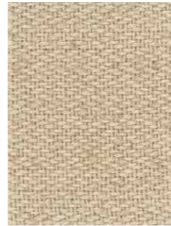
No. 15 経糸, 緯糸: バナナ50%×綿50% 混紡糸 warp, weft: 50/50 banana/cotton blended yarn
