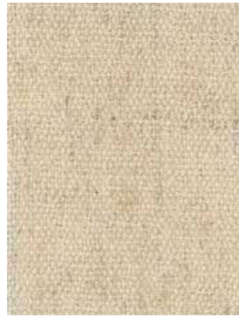
No. 6 経糸, 緯糸: バナナ50%×綿50% 混紡糸 warp, weft: 50/50 banana/cotton blended yarn
