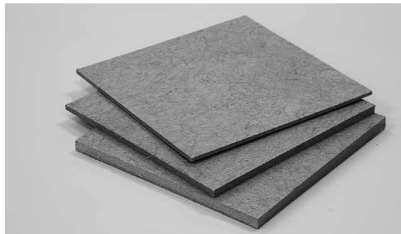
図 | Fig.27 バナナボード Banana boards made of banana and heat-adhesive fibers
