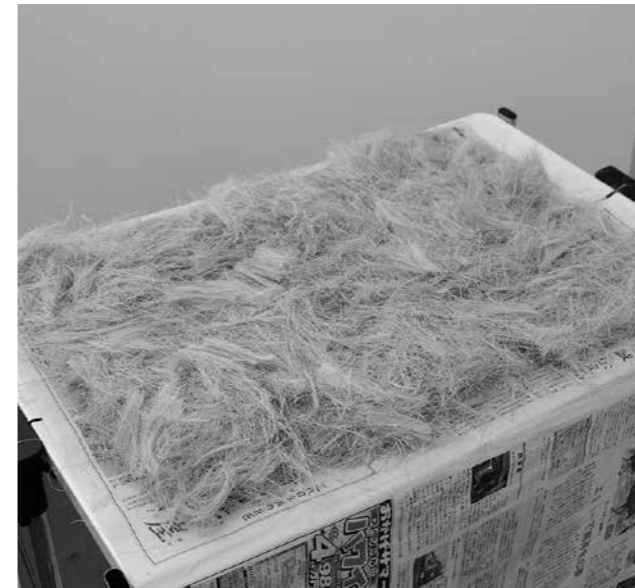
図 | Fig.28 バナナ繊維(5cm程度にカット) Cut banana fibers into approximately 5cm
