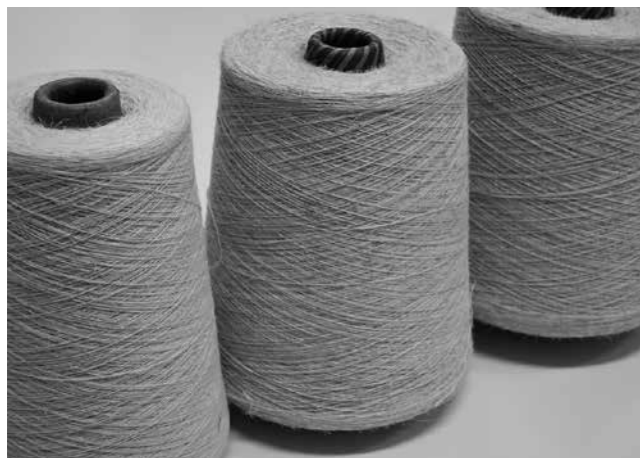
図 | Fig.17 バナナ繊維と綿の混紡糸 Banana and cotton blended yarn
