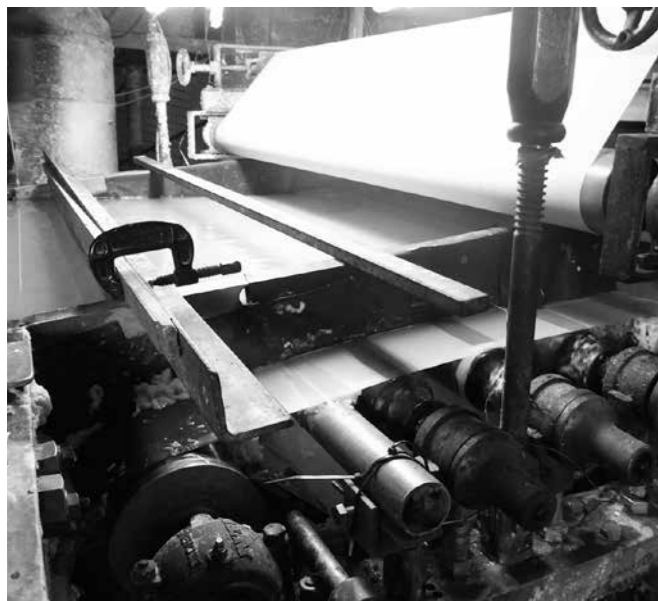
図 | Fig.40 バナナペーパーの機械製紙 | Steps of producing banana paper by machine
