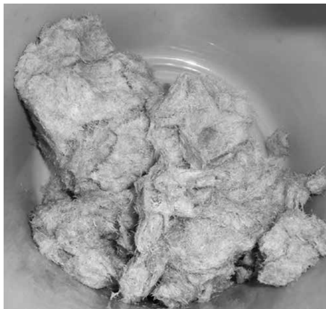
図 | Fig.38 水洗後のバナナ繊維 | Rinsed and squeezed a mass of banana fibers
